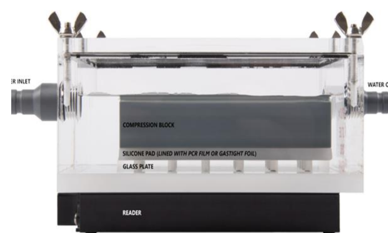
Fig 1. The Loligo Microplate System used for analysis of sirtuin inhibition in Mytilus californianus . Two of these well plates were used for respiration data collection
