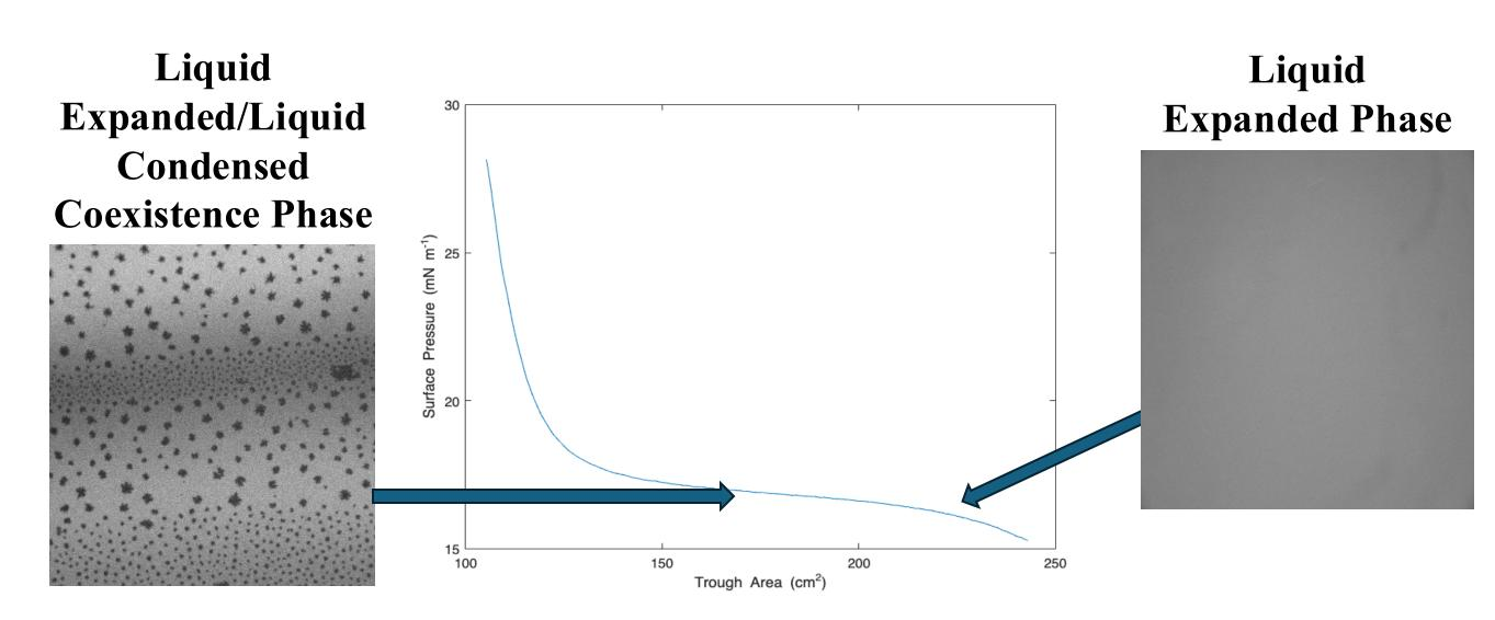
Isotherm at 23 °C of heneicosanoic acid compressing through the L2 -> LC phase transition.
