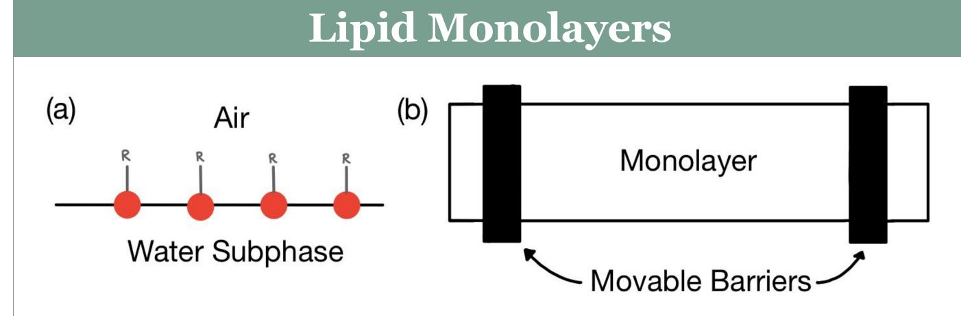
(a) Single layer of lipid oriented into a monolayer along a nanopure water subphase. (b) Top-down schematic of Langmuir trough with movable barriers to adjust surface area.
