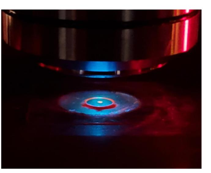
The entire film (3 mm in diameter) is shown, drawn across a circular hole in a thin glass slip.
